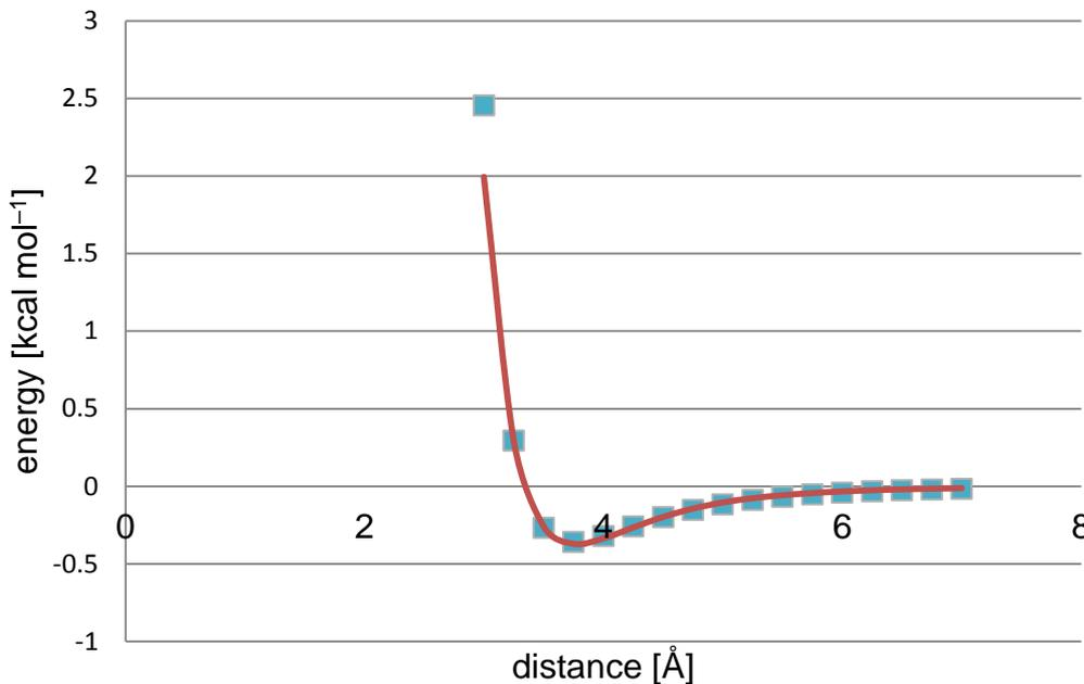
$$E_{\text{vdW}}(r) = 4\varepsilon \left[ \underbrace{\left(\frac{\sigma}{r}\right)^{12}}_{\text{斥力項}} - \underbrace{\left(\frac{\sigma}{r}\right)^6}_{\text{引力項}} \right]$$
