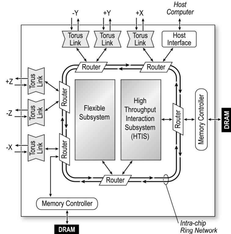
Figure 2: Anton ASIC block diagram.
