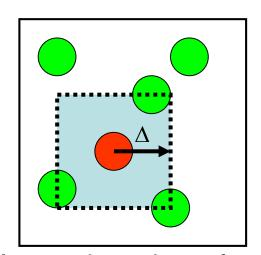
2. If the energy of the destination state,  $e_j$ , is lower than that of the original state,  $e_i$ , accept the movement. If not, accept it with the following probability:
